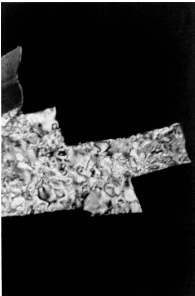
FIGURE 2 Photomicrograph of S_C - M_I transition at 141.5°C on heating [Ag(8-OPhVPy)][DOS]. See Color Plate III.
